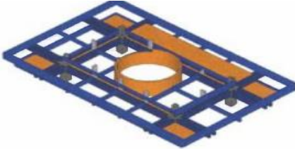
SEQUENCE 5 – REMOVE MORE UPPER PC BEAMS
